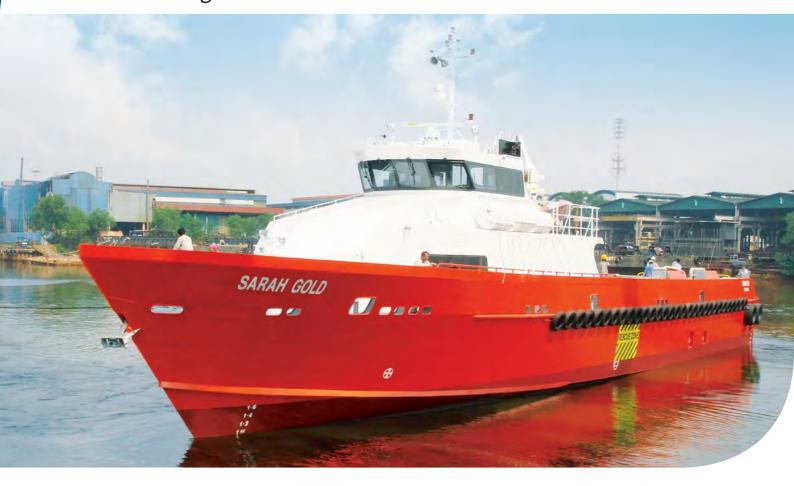
**Sarah Gold** is specially designed and built to provide high speed crew and cargo movement for Oil and Gas Exploration and Production Operation offshore. Featuring optimised deck cargo carrying area, the all aluminium constructed hull is also specially designed for the comfort of passengers.
